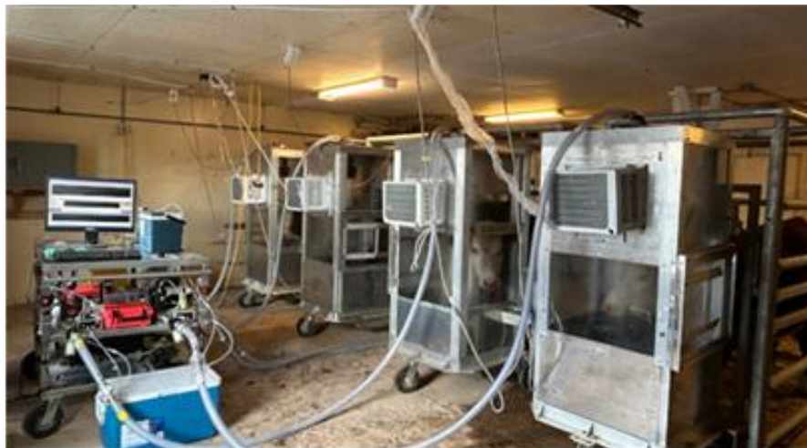
Four of the beef heifers in the measurement chambers. John and his team use these chambers to measure the output of methane.
